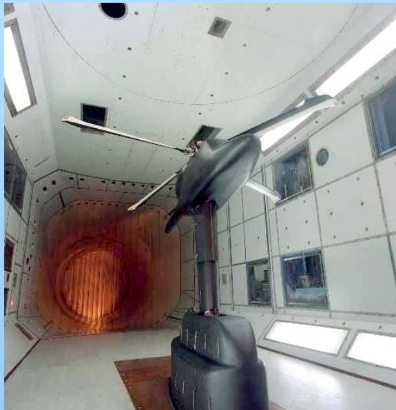
Rotor test rig and experimental rotor in QinetiQ 5 metre wind tunnel
